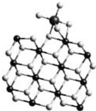
Figure 4. The 5-fold Ti configuration obtained by simulation of \text{TiCl}_4 deposition on a \text{MgCl}_2 (110) surface as described in the text.
